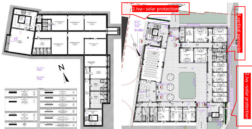
Figure 8 Phase III CAD drawings, concept Dițoiu Nina-Cristina 9 - Plans for basement, ground floor/10/final version: no more 1. Solar fireplaces and 3. Water pool on the interior court; 6. Metal horizontal sun shading (Metallic structure that support photovoltaic panels); contracted : 2. Ivy on a metallic frame – solar protection; Vertical shading system – West orientation; 5. Cantilevered terrace south orientation –
