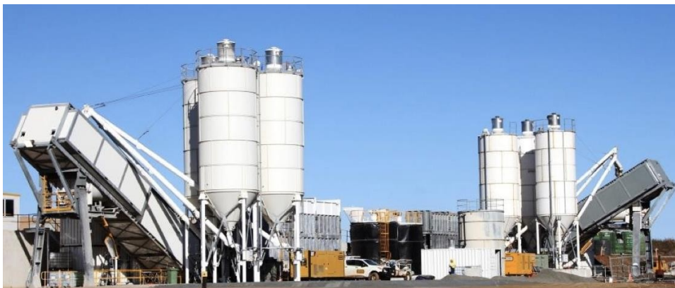
Figur 9: Geopolymer twin batch-anlegg (Glasby, Day, Genrich & Aldred, 2015)
