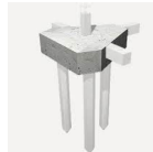
(1) Piles and pile caps
