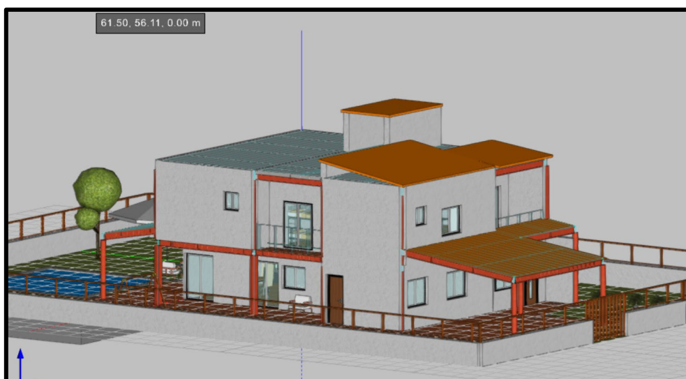
Figure 2. House with steel structure.
