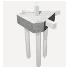
(1) Piles and pile caps
