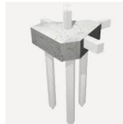
(1) Piles and pile caps
