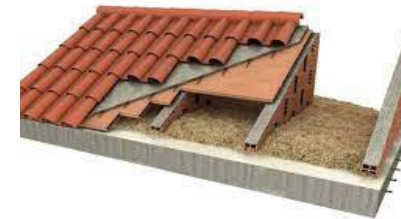
5.B - Tiled roof Tiled roof with brick walls
